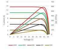
Current-Voltage & Power-Voltage Curves (580W)
