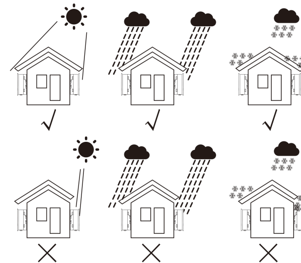
Figure 4.1 Recommended Installation locations
